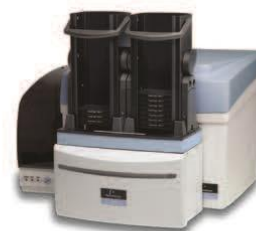
Options include a 2-channel dispenser with stirred/heated reagents reservoir for flash luminescence, calcium and other kinetic assays, and 20- or 50-plate stacker with restacking function for slow kinetic assays. Magazines are compatible with PlateStak™ automated microplate handler.
